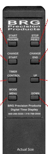
Timer - Press once to Stop, Press again to reset. Counter -Press once to reset.
