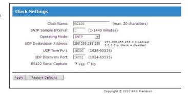
Clock Name - is the user defined name used to identify the device during a network search.
