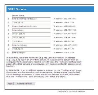
Server Name – enter the numeric IP addresses or alphanumeric named addresses of the desired network time servers. The default configuration includes ten government time server addresses.
