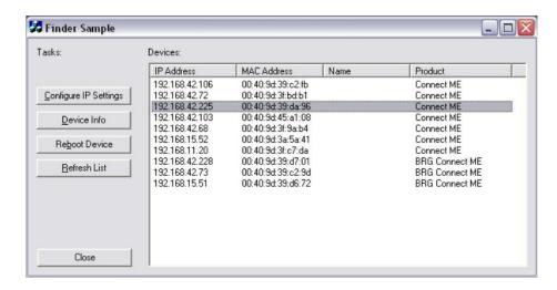
The finder exe program is a software tool that can be used to locate the Ethernet interface just about anywhere on the local network. However, it cannot be used to configure the interface. Compare the MAC address on the product label with those listed on the finder exe program. If there is a match, then the IP address will be listed next to it.
