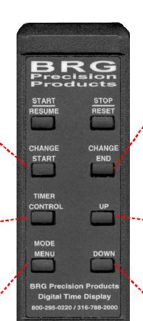
Target Hours:Minutes – Press once to access hours:minutes. Press Up or Down to change. Press again to exit.
