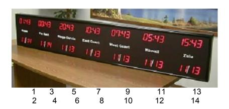
if your time zone clock has multiple rows and columns you will need to determine the actual display numbering for your clock by using the special diagnostic mode 6 which will cause the displays to show their display number instead of their normal time or date display. In examples shown below, the first display is usually the upper left or the center display.
